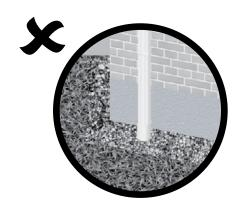
**Don't** connect your gutters to a foundation drain.
