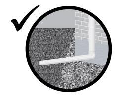
**Do** send water towards permeable surfaces, or install a rainwater recovery barrel, making sure that overflow is directed toward a permeable surface.
