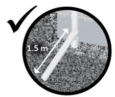
**Do** extend output 1.5m away from foundations to prevent erosion.
